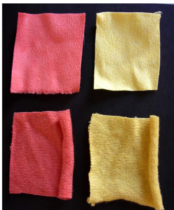
Figure 1. Polyester (upper row) and wool (lower row) dyed with 4a (left) and 4b (right).
