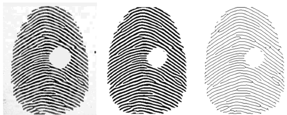
Fig. 2 Schematic of preprocessing pipeline. From left to right: original (incomplete) fingerprint image, fingerprint image after gabor enhancement, fingerprint image after thinning
