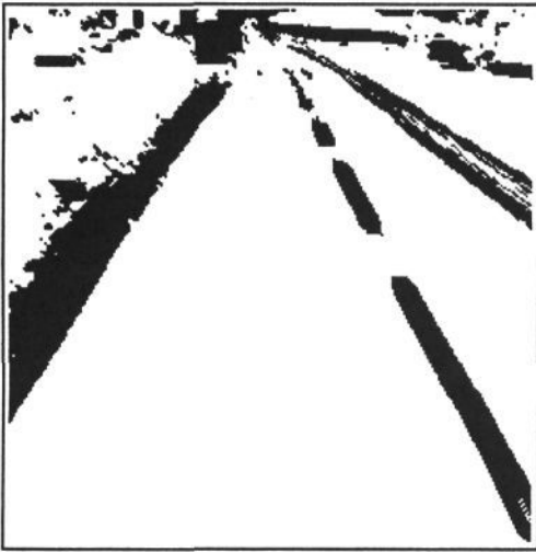
Figure 5: Edge Detection using the Covariance Filter
