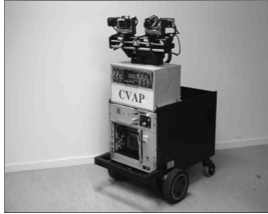
Figure 1: The experimental platform. The KTH head-eye system mounted on a mobile platform.
