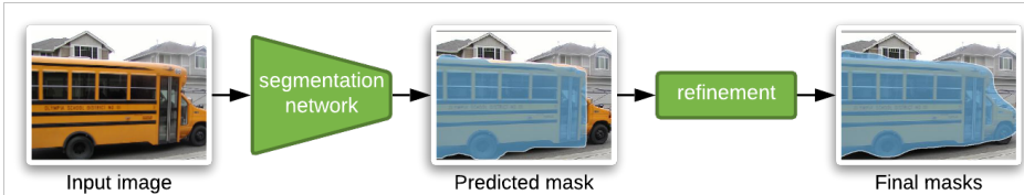
Figure 3: Inference. At test time, only the trained Mask-RCNN is required to output the prediction masks in the image. As an optional refinement step, the predicted masks can be replaced with the object proposals of highest Jaccard similarity.
