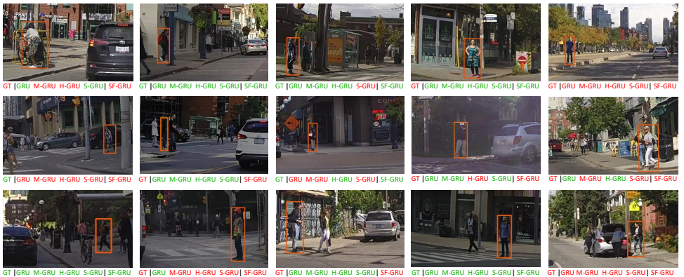
Figure 3: Examples of the predictions produced by the proposed algorithm SF-GRU and top competing methods, namely GRU , M-GRU , H-GRU , and S-GRU . In the examples, GT stands for ground truth and green and red colors indicate whether the pedestrian will cross in front of the ego-vehicle or not respectively. The instances where the color of the algorithm labels matches the GT means that their predictions are correct.
