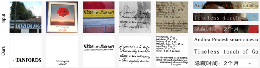
Figure 1: Top: original document images. Bottom: binary result images generated with our proposed method.
