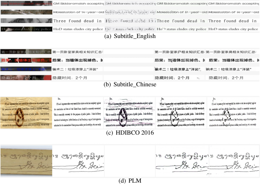
Figure 5: Qualitative results of comparing a few state-of-the-art methods on several datasets. From left to right: text image (input), ground truth, cycleGAN [65], Pix2Pix [8] and DB-RAM. The cycleGAN [65] results in Fig.5 (b) and Fig.5 (d) are totally white.
