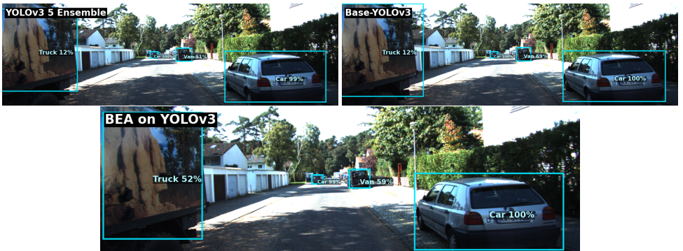
Figure 13: Exotic visual example of BEA on YOLOv3: The truck with a nature poster lowers the confidence score of the prediction in non BEA models.
