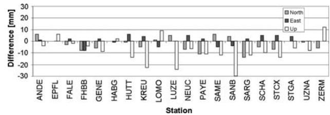
**Fig. 15** Discontinuities in the coordinate time series due to the replacement of the antennas at 20 AGNES sites
