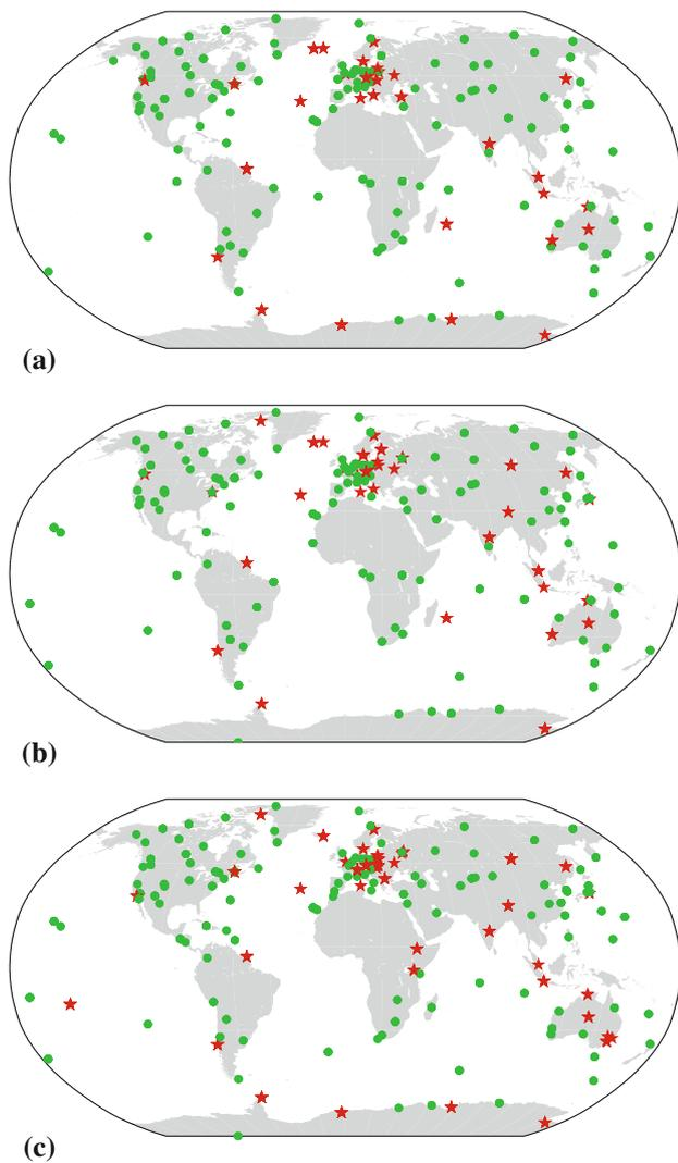
**Fig. 2** Geographical distribution of multi-system GNSS receivers (*red stars*) and GPS-only receivers (*green dots*) that are used for the CODE final processing. **a** GNSS subnetwork of the IGS in July 2003 (day of year 182). **b** GNSS subnetwork of the IGS in March 2005 (day of year 075). **c** GNSS subnetwork of the IGS in April 2008 (day of year 110)
