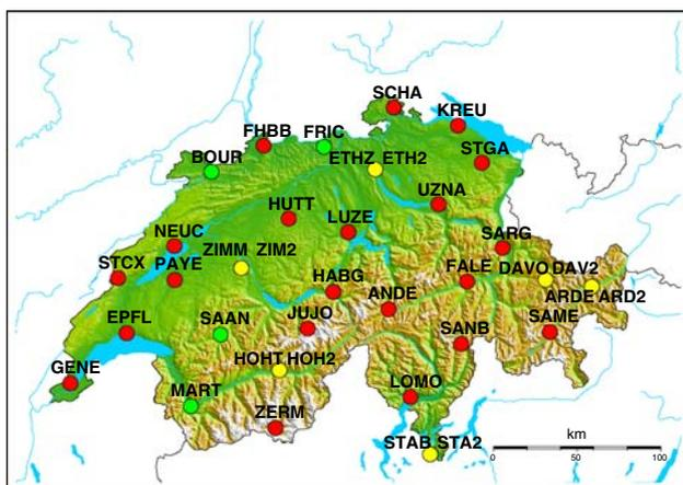
**Fig. 14** Status of the AGNES network (April 2008): red circles indicate new GPS/GLONASS receivers, green circles show the locations of stations with a GPS-only tracking receivers, yellow circles represent stations where a GPS-only and a GPS/GLONASS receiver are operating simultaneously
