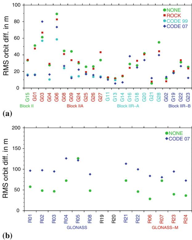
**Fig. 3** RMS differences between estimated orbits (“ground truth”) and predicted orbits based on different radiation pressure models. The orbit predictions time span was 2 weeks. Eclipsing satellites are excluded from the differences. **a** GPS satellites. **b** GLONASS satellites
