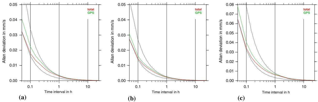
**Fig. 11** Allan deviations of the kinematic positions (at 3-min intervals over 60 days) of the combined GPS/GLONASS receiver in Zimmerwald (ZIM2) using only GPS measurements (*green line*) and observations from both GNSS (*red line*), respectively. The unusual non-logarithmic
