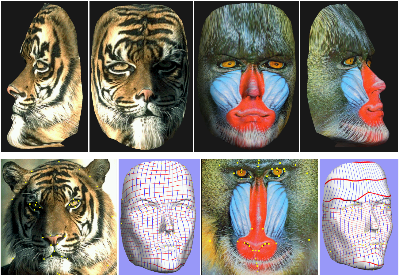
Figure 12: Mapping two different images onto the Face data set. The texture and iso-parametrics are shown for both. As can be seen, the mapping smoothly interpolates and extrapolates the feature points. (total session time : 5 min. for each)
