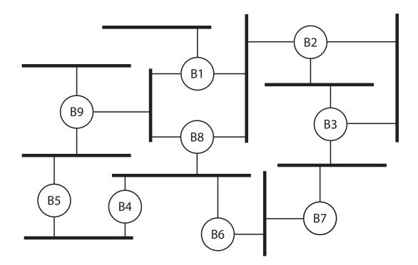
Indicate which ports are blocked by the bridge spanning tree protocol by putting an " $\mathbf{X}$ " over the corresponding ports. The bridge IDs are the numeric values. Feel free to label the ports with port numbers, if necessary. (15 pts)
