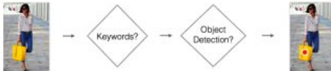
Figure 3: Instead of running all object detectors on all images, we first predict the image categories using textual metadata, and then apply object detection modules specific to the predicted category.
