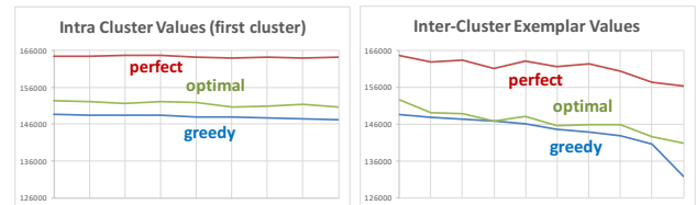
Figure 3: Intra- and inter-cluster variability. Note the strong correlation between the greedy and optimal solution within a cluster; it suffices to run the MIP on the layout with the best greedy value within a cluster. The correlation is less strong between clusters, because of the qualitatively different geometric differences between the greedy and optimal solutions from one cluster to another. For example, for the 4th cluster, the greedy solution is optimal, while for other layouts there are significant gaps. Hence it is worthwhile running the MIP on the exemplar from each cluster.
