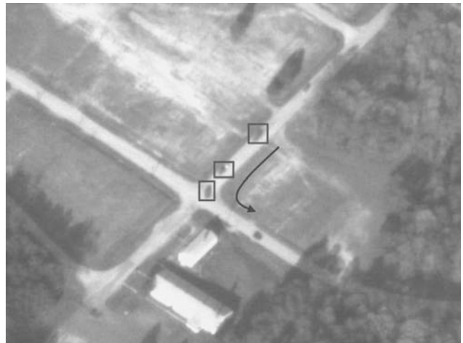
Figure 6: Convoy turning a corner. Three vehicles (highlighted) are detected as part of a CONVOY pattern.
