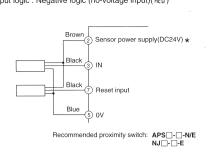
In case of a voltage output type or a PNP open collector output type
