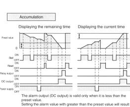
in triggering the alarm output at the timer reset value
