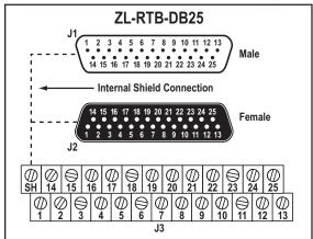
NOTE: Pinouts are straight-through, pin to pin to terminal. Example: J1, Pin 1 to J2, Pin 1 to J3, Terminal 1, etc.
