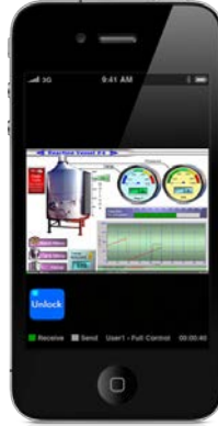
Figure 6: StrideLinx mobile VPN connectivity allows control and data viewing on third-party mobile apps, like AutomationDirect’s C-more Remote HMI.
