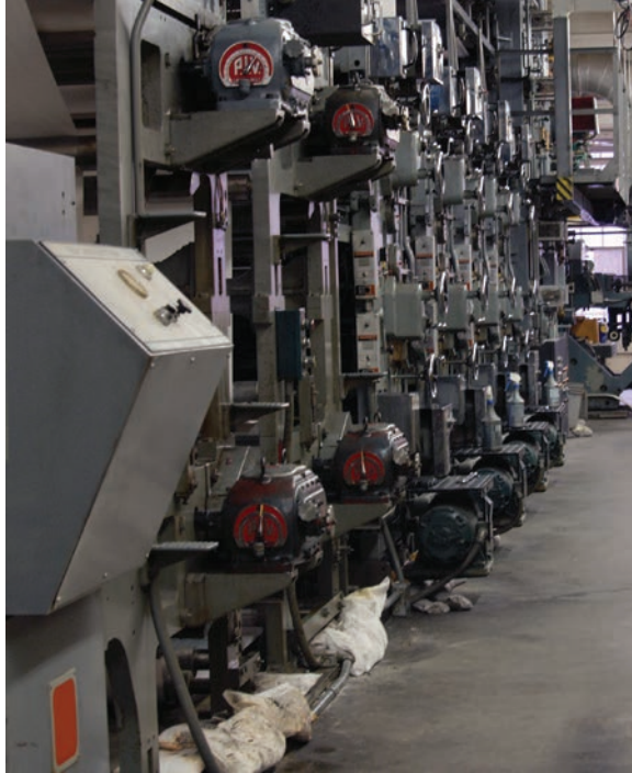
Figure 3: Web printing presses, paper mills, and material converting applications require the precise speed regulation of closed-loop control available in higher-end VFDs. Elsewhere, volts-per-Hertz (V/Hz) and sensorless (or open-loop vector) modes are used.
