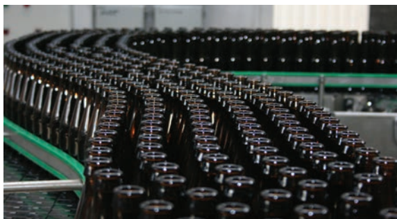
Figure 1: In addition to varying speeds, conveyor applications typically require frequent starting and stopping. Here, VFDs substantially reduce starting current to extend motor life.
