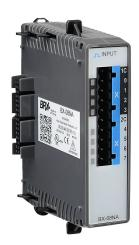
BRX discrete input module, 8-point, 120-240 VAC, 2 isolated common(s), 4 point(s) per common. Requires BX-RTB08, BX-RTB08-1 or BX-RTB08-2 terminal block kit or ZIPLink pre-wired cables.
