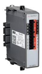
BRX relay output module, 8-point, 12-48 VDC/24-240 VAC, (8) Form A, 2 isolated common(s), 4 point(s) per common, 2A/point. Requires BX-RTB08, BX-RTB08-1 or BX-RTB08-2 terminal block kit or ZIPLink pre-wired cables.
