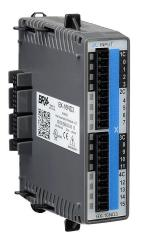
BRX discrete input module, 16-point, 12-24 VDC, sinking/ sourcing, 4 isolated common(s), 4 point(s) per common. Requires BX-RTB10, BX-RTB10-1 or BX-RTB10-2 terminal block kit or ZIPLink pre-wired cables.
