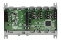
Productivity2000 I/O base, 4-slot, DIN rail or flush mount. Requires P2-01AC, P2-01DCAC or P2-01DC power supply. Holds power supply, CPU and (4) I/O modules.
