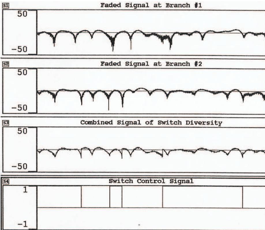
Fig. 3. Fading Signal Envelopes in Diversity Branches ( $L=2$ )
