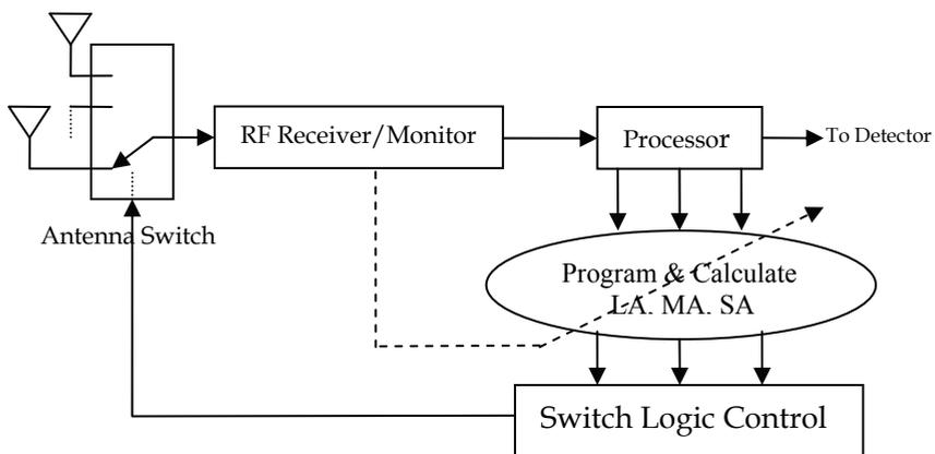
Fig. 5. Antenna Switch Diversity for Wireless Channel
