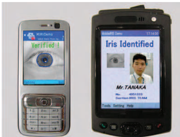
Fig. 8. Iris recognition technology for mobile terminals (OKI introduces Japan's first iris recognition for camera-equipped mobile phones and PDAs, In: OKI Press Releases , 27.11.2006, Available from http://www.oki.com/en/press/2006/z06114e.html )
