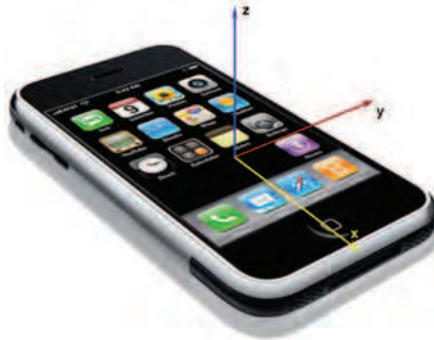
Fig. 10. Three axes of accelerometers on an iPhone (Redrawn from Tanviruzzaman et al., 2009)
