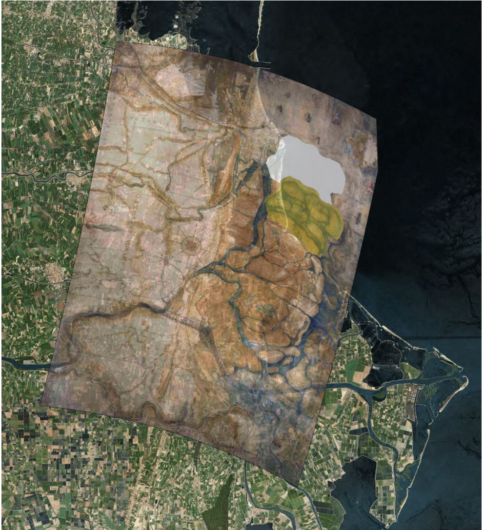
Figure 14. Overlay of the “false case”, georeferenced by means of a second order polynomial transformation, on present high resolution satellite images ( Bing Maps TM environment).
