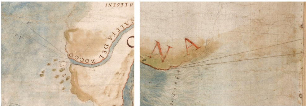
Figure 8. Examples of sighting tracks visible in L map.
