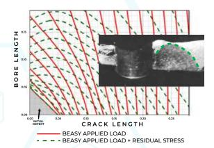
Testing validated simulations show that crack paths in residual stress fields are different
