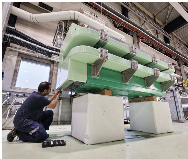
One of the East Area's magnets undergoing renovation work at CERN. (CERN-PHOTO-201903-057-9)
