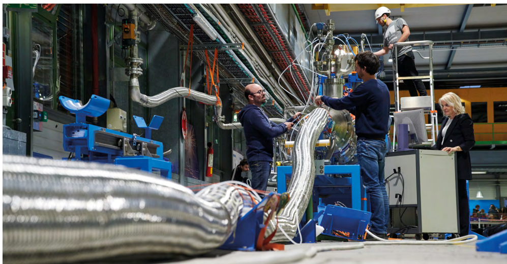
A prototype superconducting link transported up to 40 000 A. (CERN-PHOTO-201904-080-7)
