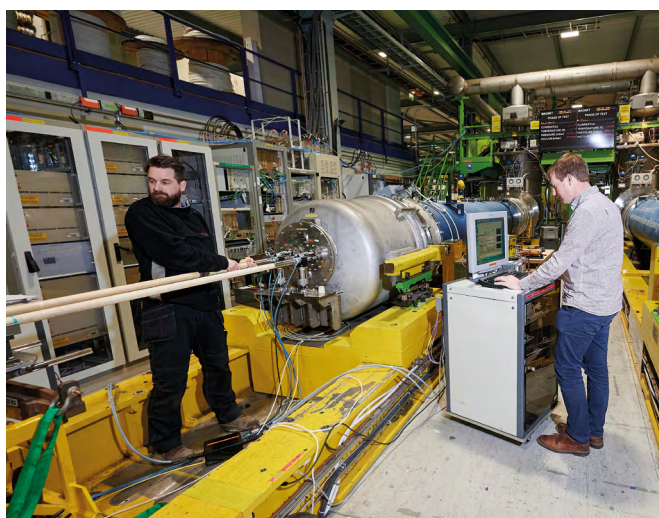
Two of the new dipole magnets using the niobium-tin superconductor, on their test benches at CERN; one of them successfully passed qualification tests in 2019.
