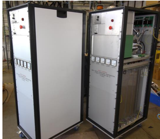
Figure 7-11: CLIQ prototype units of the second generation in the MPE test lab
