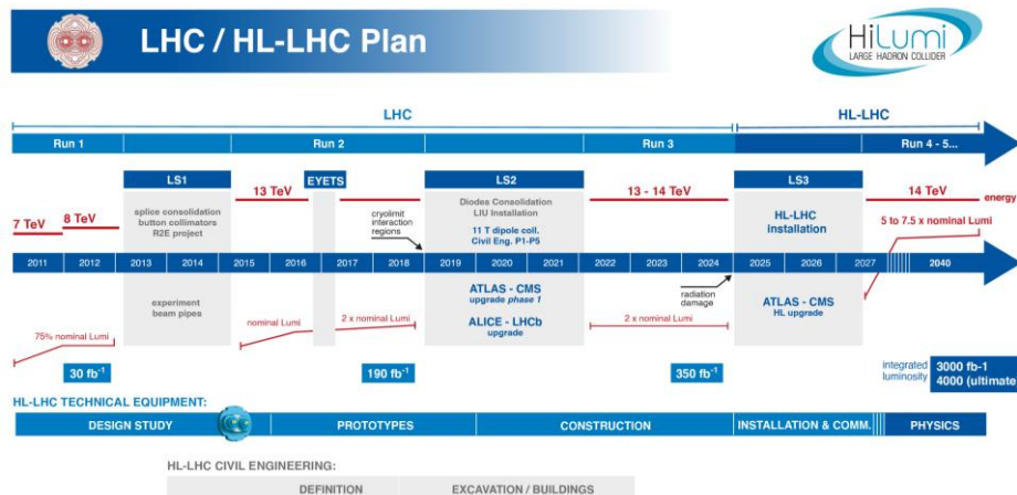
Figure 1-1: LHC baseline plan for the next decade and beyond showing the collision energy (upper line) and luminosity (lower line). LS2 sees LHC consolidation and the HL-LHC underground excavation, as well as the upgrade the LHC injectors and Phase 1 upgrade of the LHC detectors. After LS3, the machine will be in the high-luminosity configuration. Covid-19 restrictions have led to the shift of the start of Run 3 to February 2022 while the start of LS3 is maintained at end of 2024.
