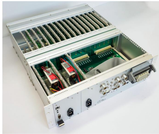
Figure 7-5: UQDS v2.1 crate serving as the baseline prototype for the 11T quench detection system. The crate is not equipped with top covers to illustrate its construction.
