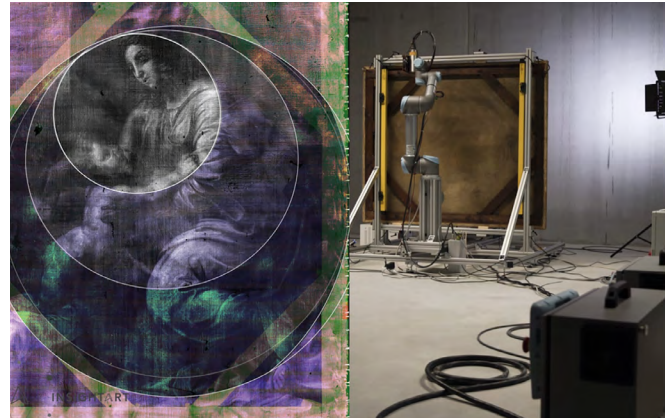
Above left: Graphic combining energy spectra measured by the RToo scanner. Above right: RToo scanning the painting The Madonna and Child.
