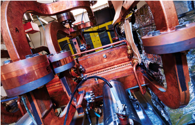
Close-up of Compact Linear Collider prototype technology, on which the future electron FLASH facility design is based. (CERN-PHOTO-202008-108-13)
