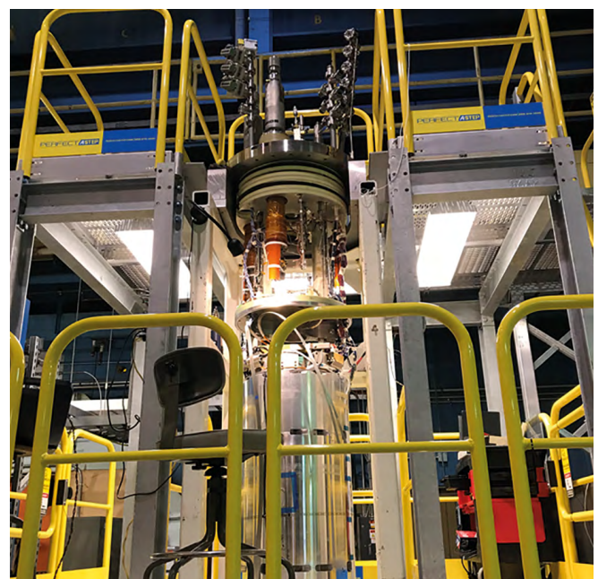
A niobium–tin quadrupole magnet for the HL-LHC project achieved a peak magnetic field of 11.4 T during a test at Brookhaven National Laboratory, in the United States.
