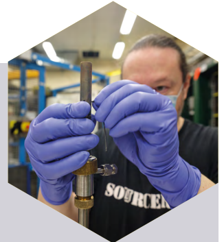
The Linac3 micro-oven is closed after being refilled with lead.
