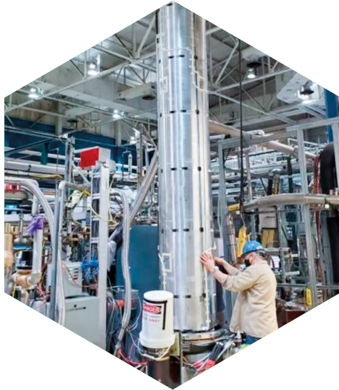
A new quadrupole magnet "MQXFA05" is tested at the Brookhaven National Laboratory, in the United States.
