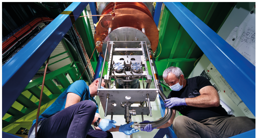
A Double-Quarter wave cavity at CERN. This technology was successfully tested at the SPS in 2021.
