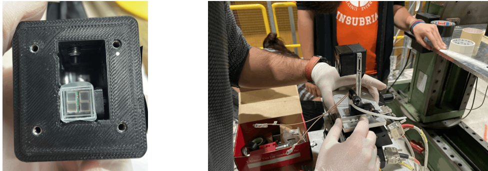
Figure 61: Left: Single crystal read out with 2 \times 2 matrix of four 4 \times 4 mm 2 SiPMs. Right: Installation of crystal on H2 beam line during fall 2022 KLEVER/CRILIN test beam.
