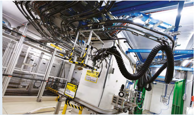
HEARTS will equip the CHARM heavy-ion facility, located at CERN, to meet the needs of the space community in testing the effects of radiation on electronic components and systems.
