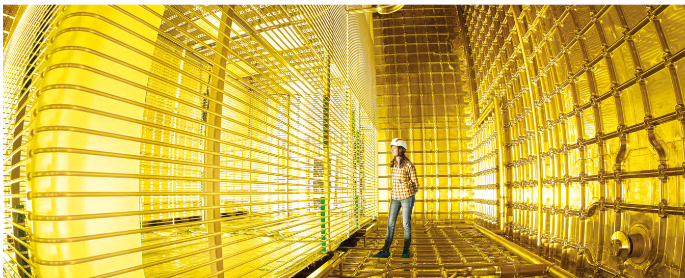
A vertical drift chamber has been installed in one cryostat of the prototypes for DUNE. (CERN-PHOTO-202308-195-28)
