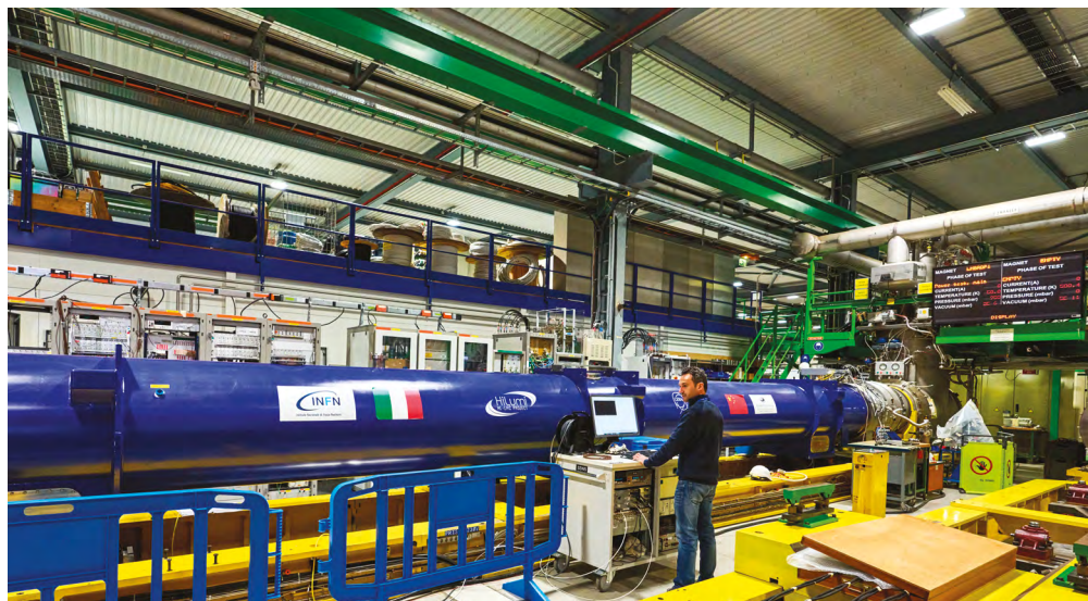
Tests at CERN of the first D2 prototype separation-recombination dipole, built in Italy by the national institute for particle physics, INFN. (CERN-PHOTO-202303-078-8)
