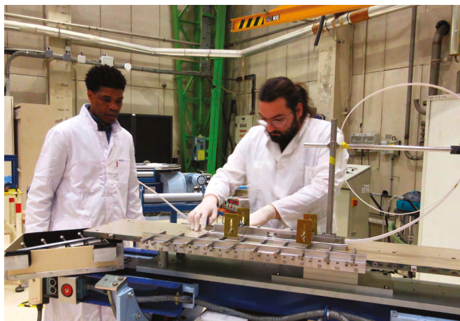
Production of a prototype coil at CEA (France) as part of the CERN-CEA collaboration for the development of niobium-tin high-field superconducting magnets.
