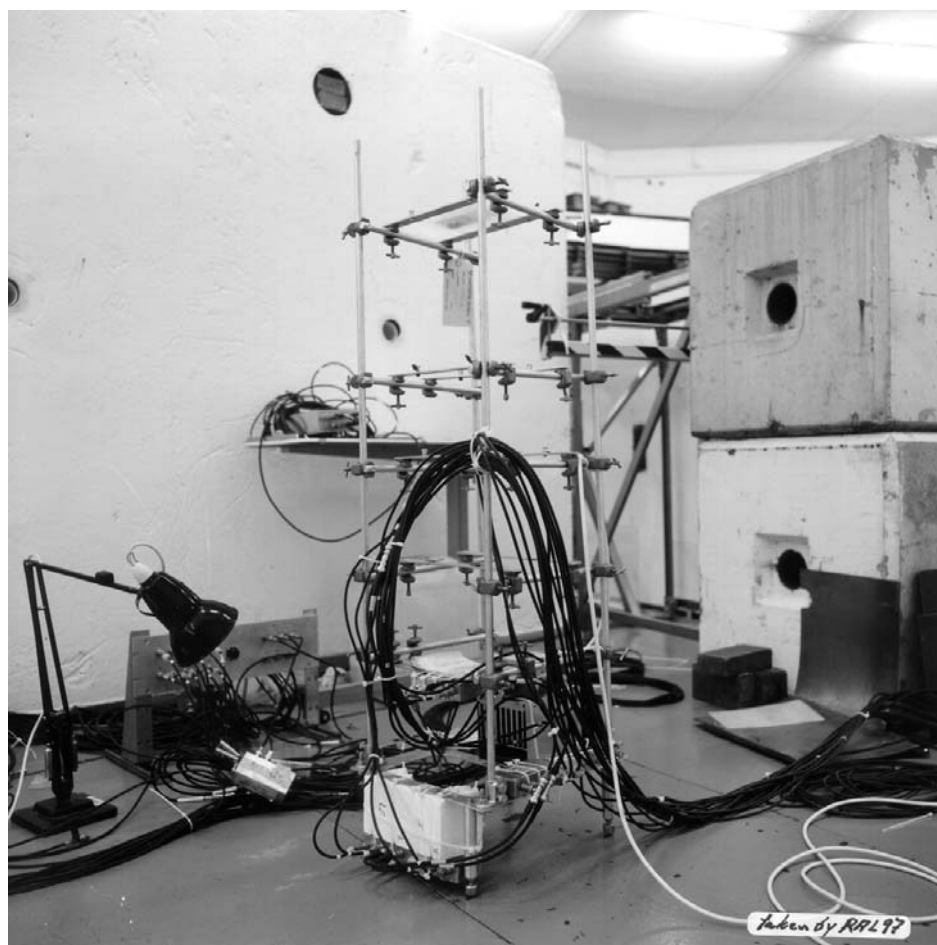
Figure 5.1: Photograph of the neutron irradiation stand. The diamonds are in boxes at the base of the stand. The picture was taken during installation of the 11/97 irradiation at ISIS at the Rutherford Appleton Laboratory (RAL).
