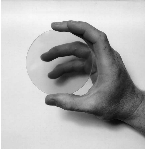
Figure 4.21: Free-standing, 100 mm diameter CVD diamond window, (courtesy of De Beers Industrial Diamond Division (UK) Ltd.) [53].
