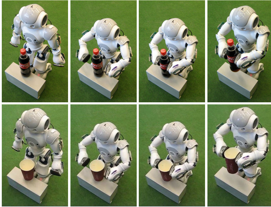
Fig. 4. Top row: robot is grasping a plastic bottle of coke with a weight of ca. 400g which requires the maximal force the robot can apply; bottom row: grasping a paper cup requires a gentle touch, a forceful grasp would deform the cup;
