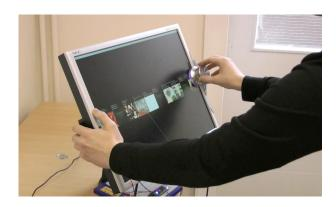
Figure 5: Users share control over an intelligent radio system, using a knob and pressure sensor.
