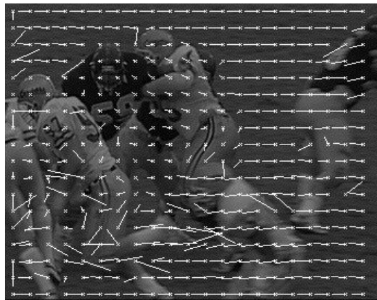
Figure 8. Motion vectors on the “futboll” test sequence
