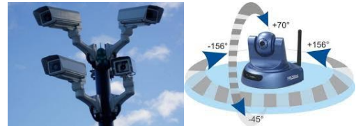
Figure 2: Examples of video surveillance cameras having the same position but different fields of view
