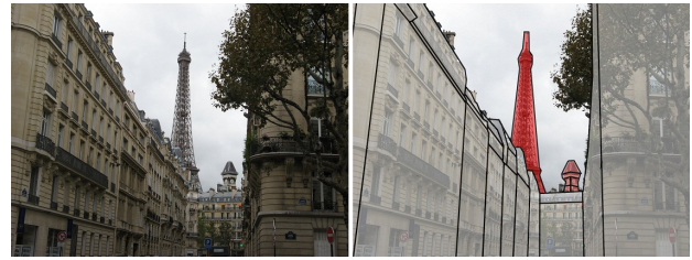
Figure 2: A representation of the ARCAMA-3D application. (a) on the left: real view (b) on the right: a 3D model of the surroundings is overlaid on the real view with 'red' objects indicating some interactive objects providing access to information.
