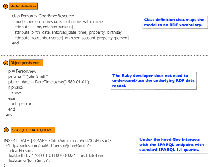
Fig. 1. The top of this figure is an example of a Goo model definition. The settings in this model establish object validations and how this model is represented in RDF. For more details on each of these settings see the project documentation page at http://ncbo.github.io/goo/ . The second part of this figure is a script that shows how we achieve persistence like similar ORM-alike libraries.
