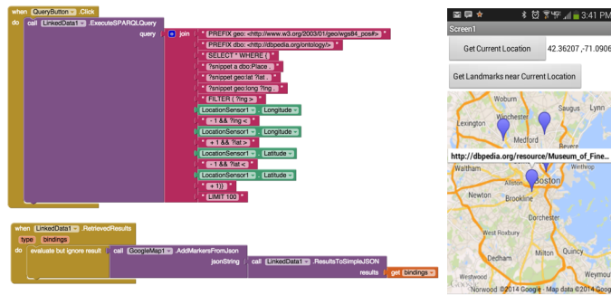
Fig. 1: Consuming Linked Data. Left: Logic used for obtaining the user’s location, constructing a SPARQL query, querying a remote endpoint, and displaying the retrieved results on a map. Right: Output as seen on the phone. ‘QueryButton’ in the blocks editor is the name of the button with the label ‘Get Landmarks near Current Location’ as seen on the phone.
