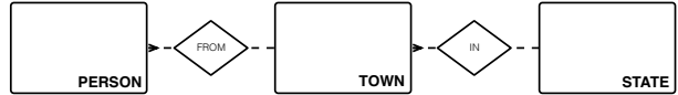
Figure 4: Relational schema that depicts a hierarchy. A state has many towns, but each town is in one state, and many people are from the same town, but each person is from one town.
