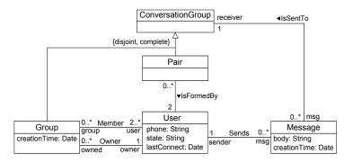
${\bf Fig.\,1.}$  Class diagram of a instant message service
