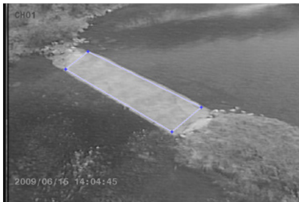
Figure 4. Definition of the vertices of a polygon to select the RoI within the substrate panel.
