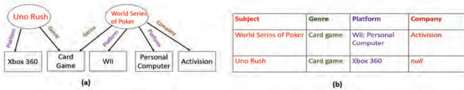
Fig. 2. The property table representation. For subjects ‘missing’ a property, the reserved keyword null is entered. ; is a reserved delimiter allowing fields to be sets .
