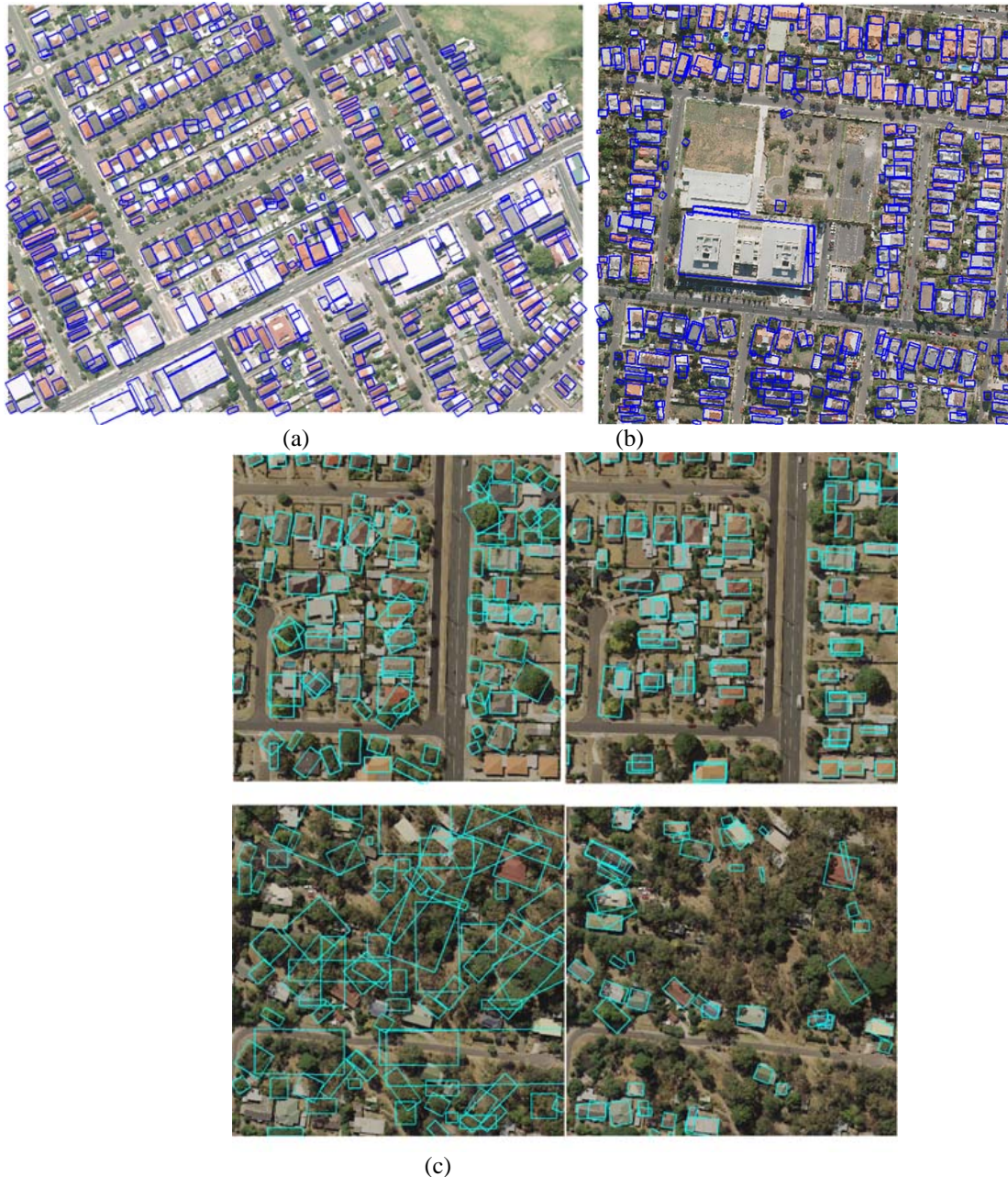
Fig. 4. Separation of trees and buildings for building detection in (a) Fairfield, (b) Moonee Ponds and (c) Knox. In (c), the detected buildings by Awrangjeb et al. (2010) on two samples are shown on the left for comparison, while the detected buildings with the methods described here are presented on the right.
