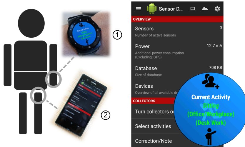
Fig. 1. Collector and labeling framework: Wear App (smart-watch, 1) and Hand App (smart-phone, 2). The positions of the devices may vary.
