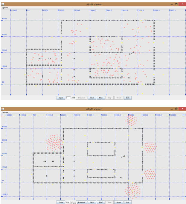
Fig. 9. Initial and final view of the simulation of a crowd evacuation.
