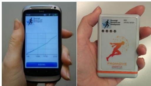
Fig. 1. The Activity Coach. Left: Smartphone (HTC Corporation, Taiwan) showing the application. Right: ProMove 3D accelerometer (Inertia Technology, The Netherlands).
