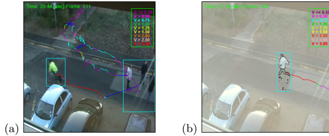
Fig. 2. (a) The low-level processing of the video. Blobs are designated by cyan rectangles; multicoloured lines denote tracks of the blobs. The program estimates the velocity of the blobs and designates it by different colours. Straight blue lines designate possible links between the blobs. (b) The wR^2 metrics is computed on the basis of temporal changes of the length of the contour of the blob.
