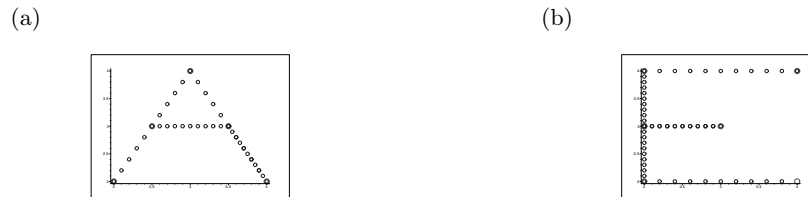
Fig. 4. Plot of the letter "A" (the control points: (2;2),(3;4),(4;2),(3.5;3), (2.5;3)) (a). Plot of the letter "E" (the control points: (4;4), (2;4), (2;3), (3;3), (2;3), (2;2), (4;2)): (b).
