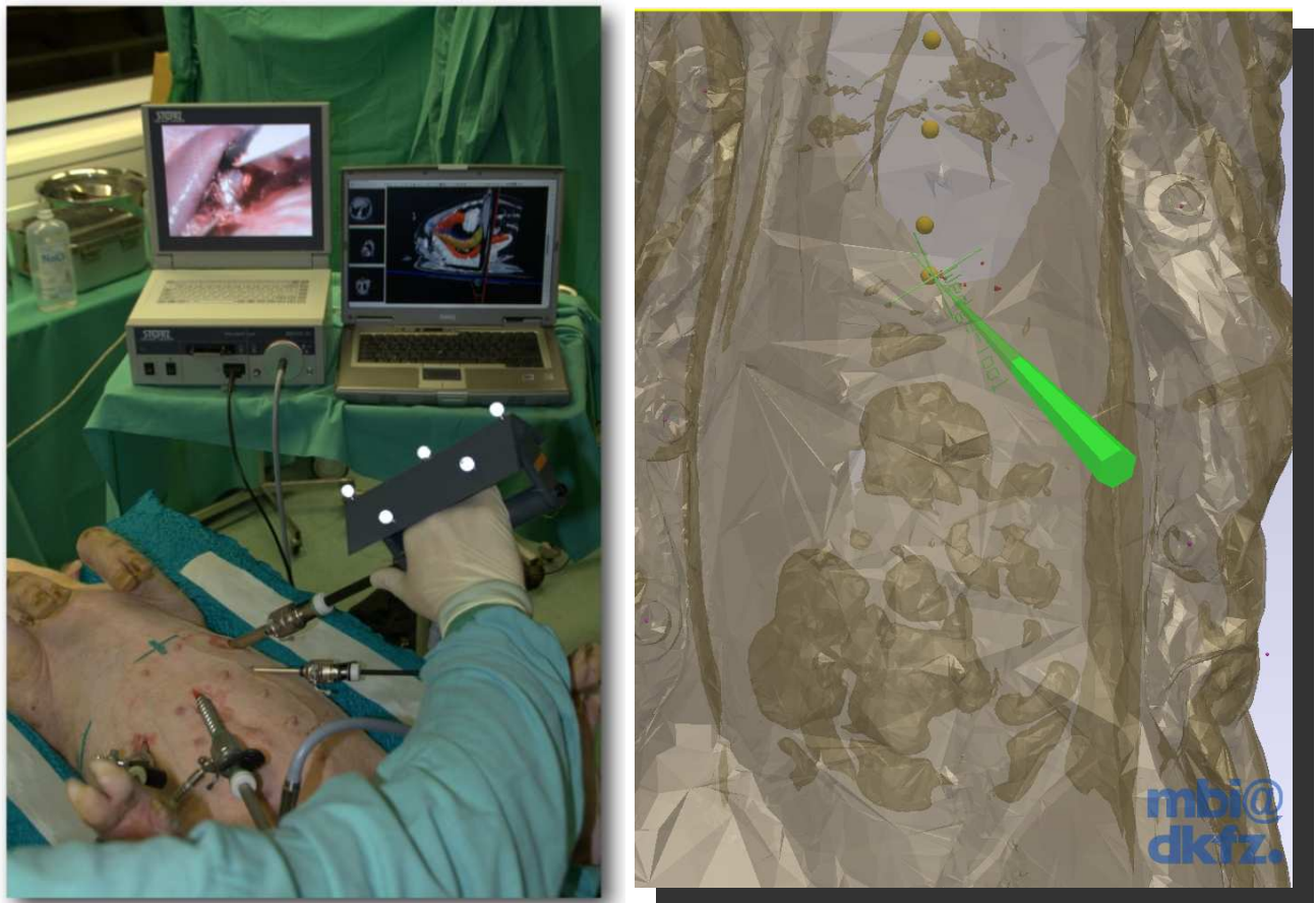
Fig. 1: Experimental Setup with the navigated instrument in the right hand of the surgeon and the Navigation System on a Laptop next to the laparoscopy unit on the left side. The instrument is displayed in the Navigation System in relation to the targets in the esophagus in real-time during the experiment.
